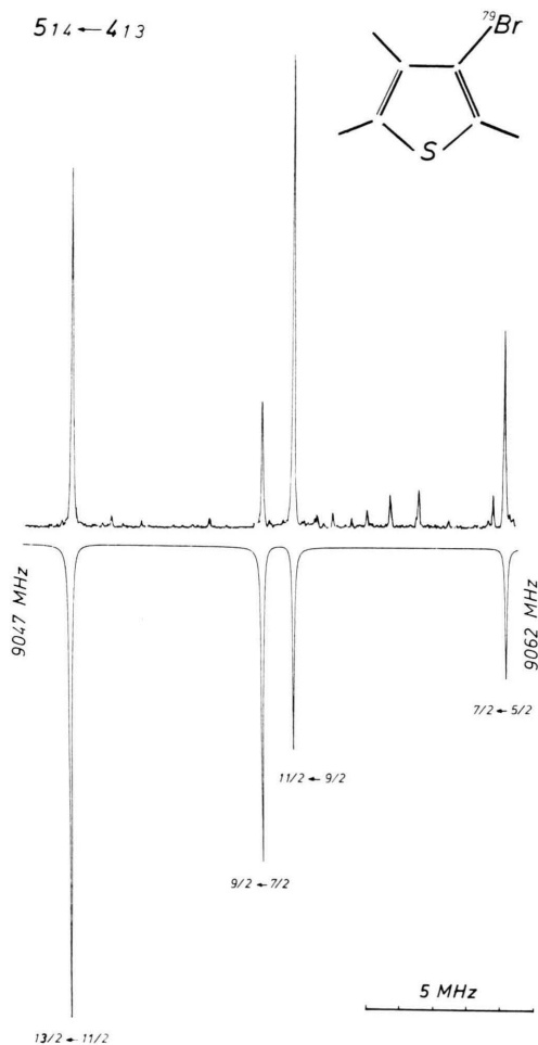
Fig. 1. The upper trace shows the power spectrum for the central section of the ^{79}\text{Br} quadrupole hyperfine multiplet of the ^{12}\text{C}_4\text{H}_3\text{S}^{79}\text{Br} 5_{14} \rightarrow 4_{13} rotational transition. The time domain signal consisted of 1024 data points taken at 20 ns per point after a delay of 0.5 \mu\text{s} to allow pulse echoes to die out. The pulse duration was 90 ns. The carrier frequency in the exciting pulse was 9057 MHz. Eight times 256 k successive free induction decay signals were sampled in order to improve the signal to noise ratio. 3072 zeros were added before Fourier transforming. Pressure: 1.12 mTorr. Temperature: -56^\circ\text{C} . The lower trace shows a computer simulation calculated according to Eq. (1) from the quadrupole coupling constants, rotational constants and centrifugal distortion constants listed in Tables 3 and 4. The experimental linewidth is 80 kHz full width at half height. „Wrong“ relative intensities in the experimental spectrum are partly due to the frequency-offset dependence of the polarization efficiency of the pulse.
